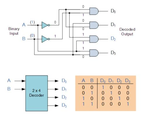
In this simple example of a 2-to-4 line binary decoder, the binary inputs A and B determine which output line from D0 to D3 is "HIGH" at logic level "1" while the remaining outputs are held "LOW" at logic "0" so only one output can be active (HIGH) at any one time. Therefore, whichever output line is "HIGH" identifies the binary code present at the input, in other words it "de-codes" the binary input
